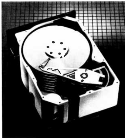
Maxtor's new 5 1/4" Winchester has 140M bytes on eight plated disks.
