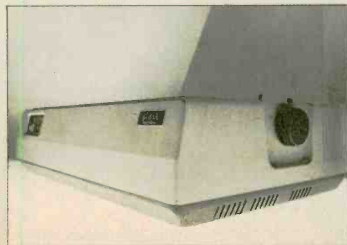
ML-83A: All the features of the 82A, including double-width and bold characters. The 136-column-wide carriage can handle paper up to 16 inches wide.
