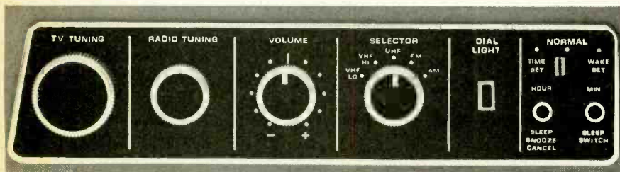
Controls for the TV and radio tuning, volume and function selections are on the side of the cabinet.
