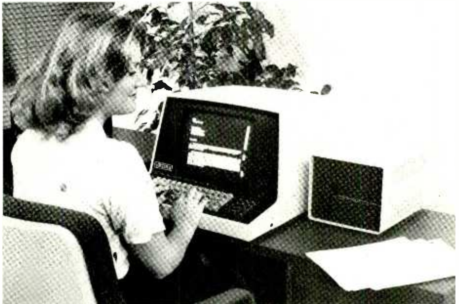
Vector Graphic's 3005 word and data processing system has 5-MB 5¼-inch Winchester disk and one 630-KB floppy disk for expanded capability.
