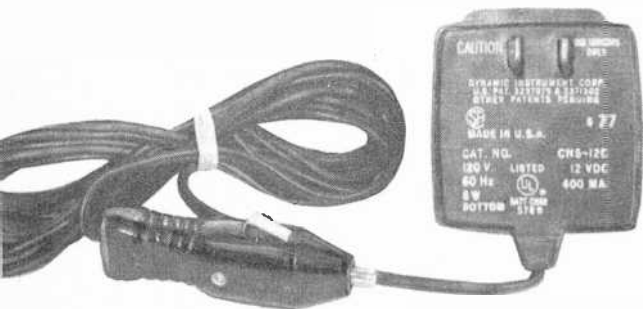
Ac adapter used as a trickle charger for automotive battery.
