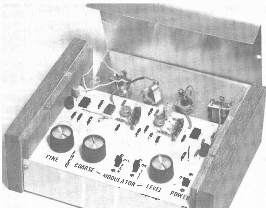
Photo of author's prototype shows how pc board extends under control panel to hold switches and potentiometers.
