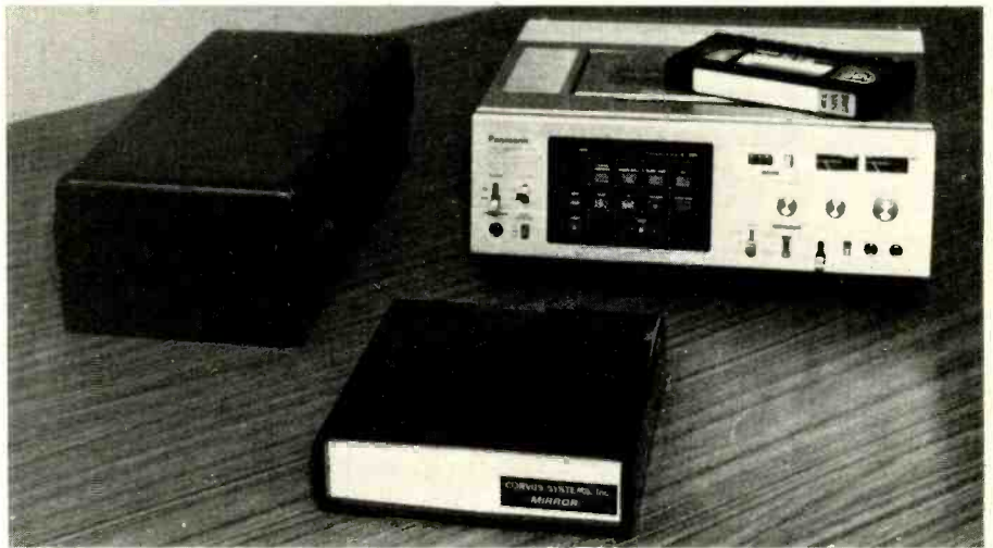
Corvus Mirror and VHS tape system provide tape backup for 8-in. drives.
