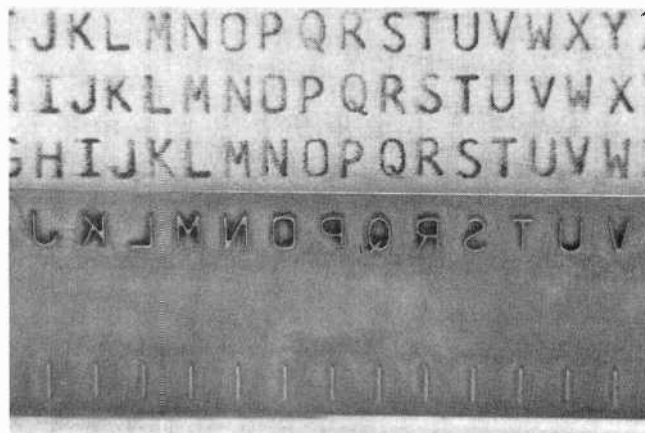
Printing band produces preformed characters but legibility is only fair to poor.
