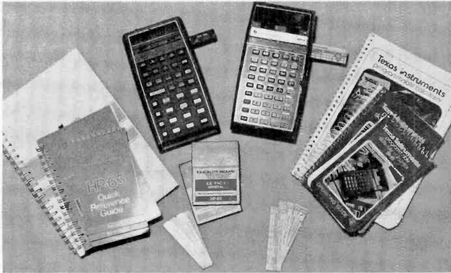
The HP-65 (left) and SR-52 are two fully programmable handheld calculators. Both incorporate a miniature magnetic program card reader.
