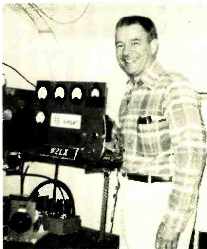
Stuart Cowan, W2LX, Rye, N.Y., and his home-constructed, 40-watt, 146-MHz transmitter. He has worked a dozen countries in three continents using the OSCAR satellites. Antennas include a 14-element Yagi, a beam, and a center-fed wire doublet.
