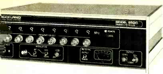
Fig. 3. Rockland Systems Model 5500 synthesizer has frequency range of 10 Hz to 40 MHz in 1-Hz steps.
