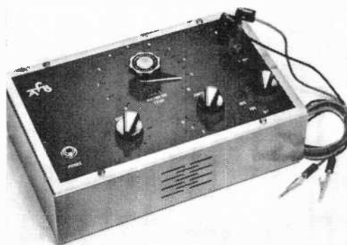
This American Foundation for Blind instrument provides tactile readings of voltage, resistance, and current. Earphones supply signal which is nulled to obtain reading.
