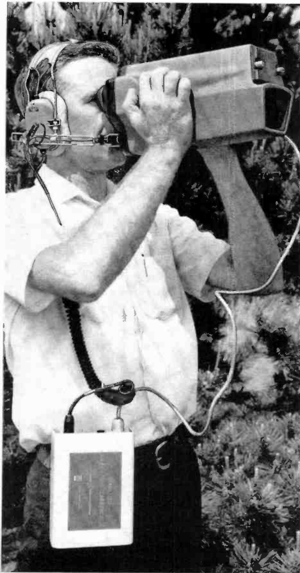
The American Laser System's Slacom laser diode communications system incorporates a novel optical technique to cancel movement effects and permit handheld communications up to about 20 miles.
