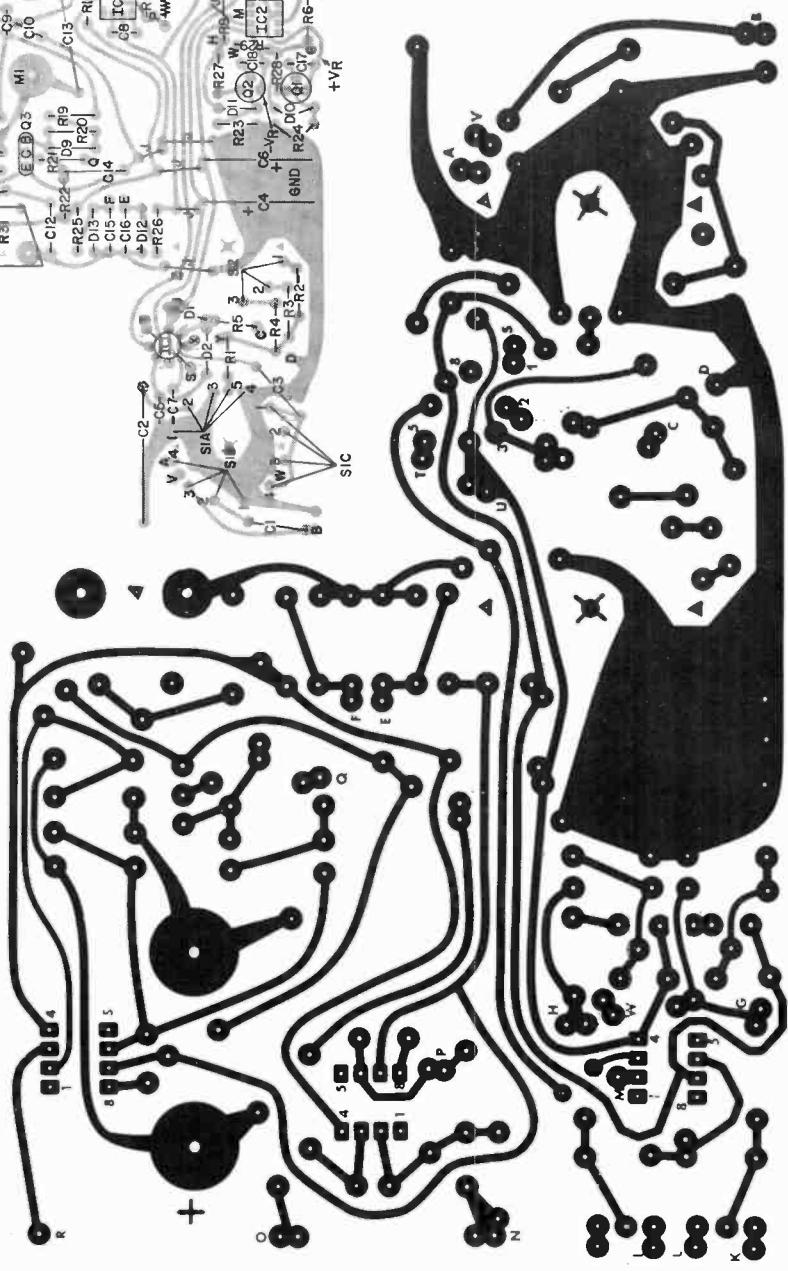
Fig. 3. Actual-size foil pattern for Super Op is below; component layout shown at left.
