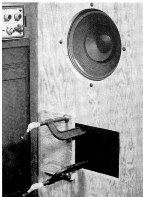
Fig. 3. Setup for running impedance curve. First calibrate variable resistance using ohmmeter and mark resistance at various settings of control knob. With equipment as shown, feed 200-Hz signal into speaker. Then, vary frequency downward, taking voltage readings at close frequency intervals. To read impedance at any frequency, note value of ac voltage on meter with switch in position S. Then switch to position R and vary knob setting to obtain the same meter reading. Record the resistance reading indicated by the exact frequencies of the peaks and valleys. Then plot the curve on a sheet of semilog paper.
