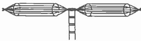
Fig. 2. Cage type of multi-wire dipole. Though a two-wire feeder is shown, this antenna can be adapted to conventional 52-ohm coaxial feedline.
