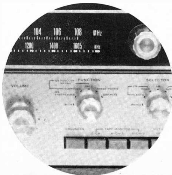
Function switch of a Sansui receiver which uses the Vario-Matrix system in its QS regular matrix decoder.
