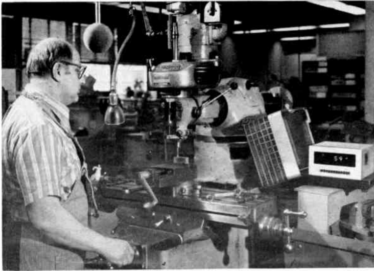
Fig. 3. Milling machine operation is monitored by General Radio 1934 noise exposure meter. Mike is in windscreen right of operator's head.
