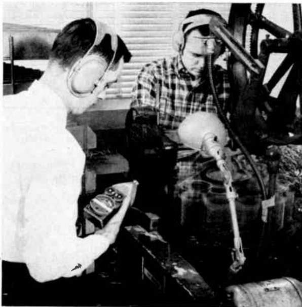
Fig. 2. Sound-level meter (General Radio 1565) being used to investigate noise produced by a braiding machine. Note protective earmuffs worn by sound surveyor and machine operator.
