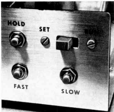
Operating controls should be clearly identified wherever they are located. Ordinary press-on type (available at all art stores) can be used for this.
