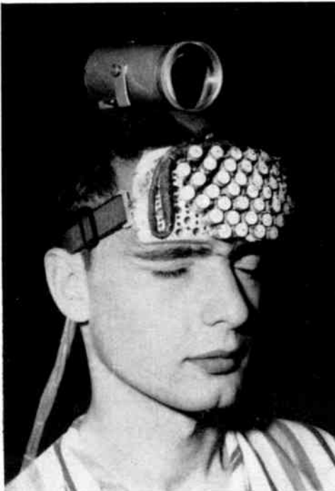
Sight is replaced by touch in the "Elektroftalm" recently developed in Poland. Image is scanned by photoelectric camera atop blind patient's head and "displayed" on forehead. Vision is rudimentary.
