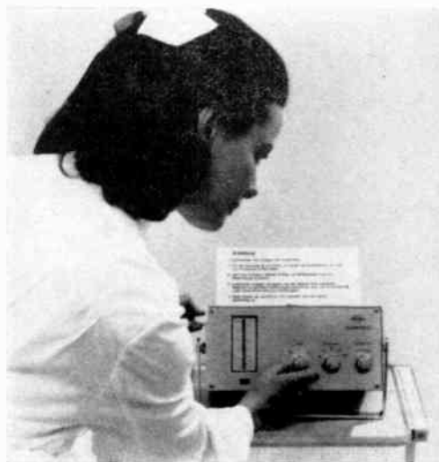
The German "Dormed" electro-therapeutic sleep inducer is not available in the USA. It generates 12-to-200-Hz square waves (15 V at 3 mA) which are applied to the patient's temples and forehead. (Photo courtesy the Robert Bosch Corporation.)
