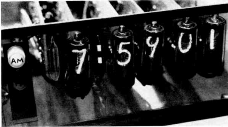
The colon is made by painting black bands on a neon lamp. If desired, another colon may be used between the seconds (the two readouts on the right) and the adjacent unit minutes indicator. In this time example, the tens hours neon is not lit.
