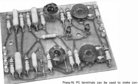
ress-int ro terminals can be used to make connections to the board. No chassis is shown here because board is designed to be mounted in an existing single-wave generator and get its d.c. power either from the generator supply or a built-in source of +18 and -18 volts. The squarer can be switched in through a switch on the front panel.
