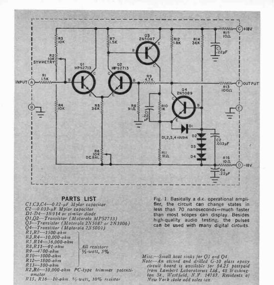
deliver 15 volts peak-to-peak into an essential open load and will trigger with any input signal of a half a volt or more.
