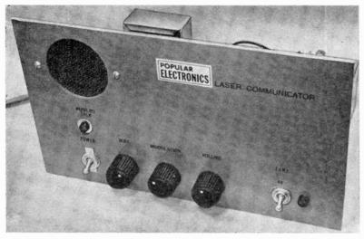
The main chassis for the telescope communicator mounts the relatively heavy power supplies (except for the laser), all controls, and is connected to the telescope electronics via a multi-lead flexible cable. Microphone plugs into the rear.
