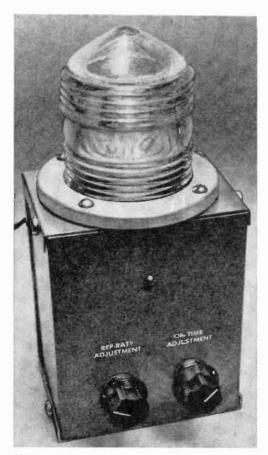
The Fresnel lens assembly bolts to the top of the chassis box with four sets of #6 machine hardware.
