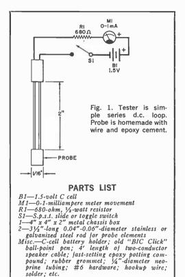
chassis mounted components. Make sure that no component interferes with the others and that the meter movement is connected with the proper polarity.
