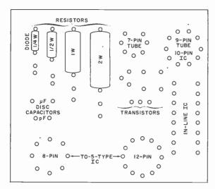
Fig. 1. Template guide, shown actual size, gives minimum hole spacing for most commonly used components. Most signal and low-current diodes fit into \(^1/4\)·watt resistor slot; other silicon diodes fit into \(^1/2\)· or 1-watt resistor slots. Eliminate one dot in upper right drawing for nine-pin tubes.
