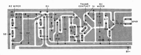
Fig. 5. Viewed from conductor side of board, foil pattern is in grey. Area etch technique was used here, but minimum-width conductor would have served just as well.
