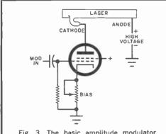
Fig. 3. The basic amplitude modulator uses a conventional pentode in series with the laser. The suppressor grid is electrically connected to the cathode.
