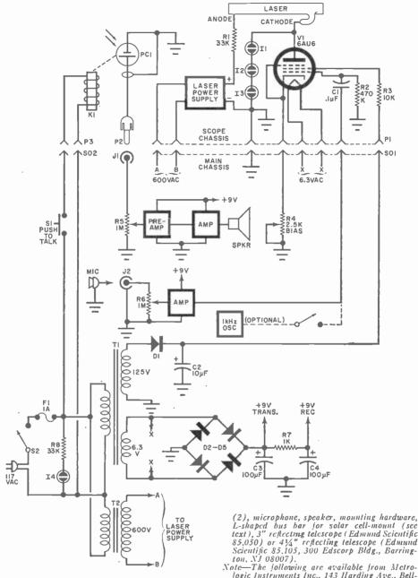
T2-Power transformer; secondary 620-650 volts at 50 mA
