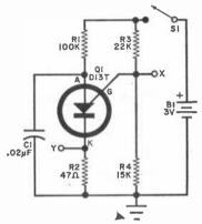
Fig. 3. Low-voltage oscillator circuit using programmable unijunction transistors has many uses.
