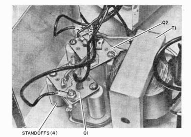
With aid of standard phenolic sockets and insulated spacers, mount transistors to rear of chassis below transformer T1 as shown.
