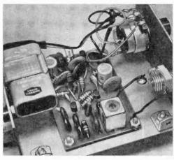
Most of electronics package is on a PC board. Use care in soldering in the 5 transistors (3 FET's). Assembly of board took your reviewer about  $1\frac{1}{2}$  hr.
