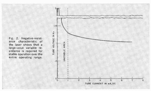
tends to turn itself off. The light output increases reasonably linear with tube current up to approximately 5 mA. Above that, the light output drops drastically and tube life is decreased. If the current is centered on the middle of the linear portion of the curve and varied about that point, the light output can be made to swing in a linear fashion and very high modulation levels can be obtained.
