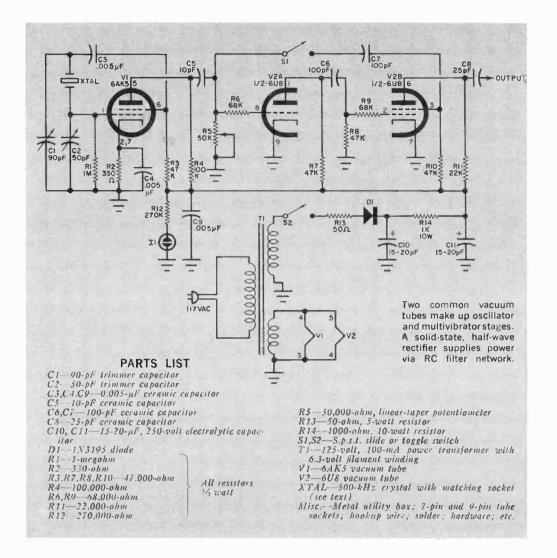
R5 set at approximately mid-range, an uncontrolled oscillation of about 50 kHz is obtained. However, by injecting the 500-kHz signal from V1 into the multivibrator, a very stable 50-kHz signal appears at the output.
