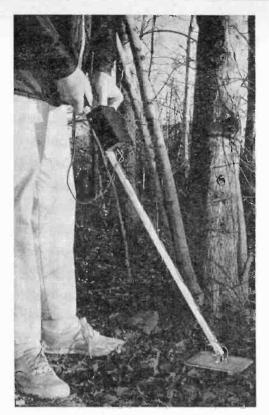
The metal/mineral locator is very light in weight and easy to use. Angle of search coil plane may be changed to suit convenience of user. Support pole is in two pieces and can be folded up into a relatively small package to fit in car trunk.
