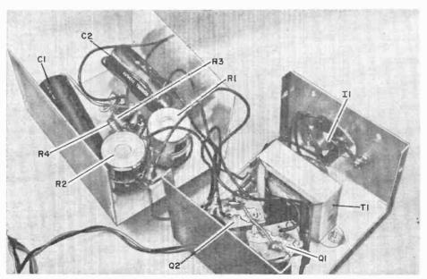
Due to simplicity of circuit, point-to-paint wiring, using stranded hookup wire, is best for assembling project. Mount controls on front, lamp and lens assembly to top of chassis box.
