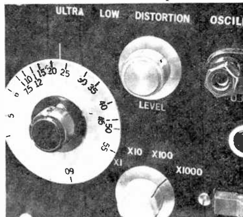
Calibration markings on sweep-frequency control dial (left in above photo) are obtained by interpreting Lissajous patterns produced by 60-Hz line and oscillator output frequencies fed into an oscilloscope.
