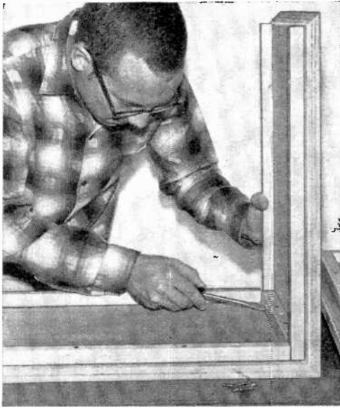
Fig. 3. Attach all cleats and glue blocks; glue and screw together top, bottom, and sides of enclosure.
