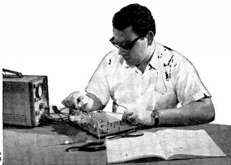
Performing transistor experiments on programmed breadboard — using oscilloscope
