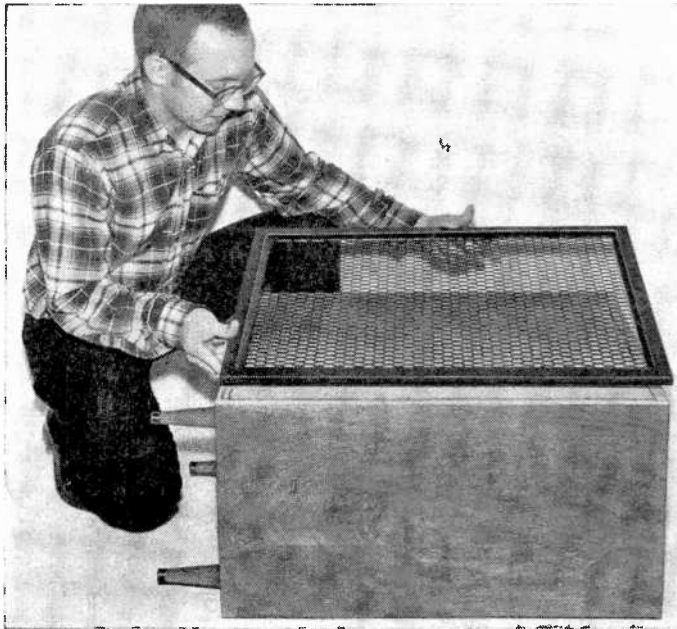
Expanded aluminum grille/picture-frame assembly goes into place only after grille cloth has been tacked onto speaker mounting board. You can use wire brads or ornamental screws to fasten the assembly down.
