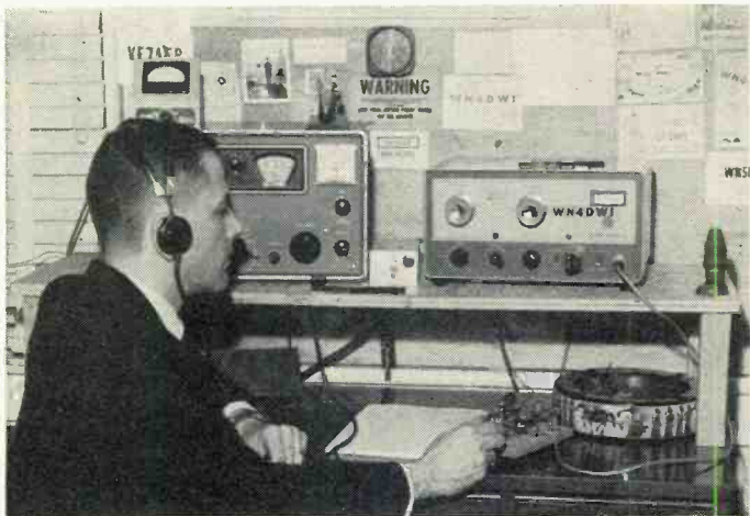
Robert Nichols, WN4DWI, has worked 37 states and a half-dozen countries with his Hallicrafters HT-40 transmitter and Hammarlund HQ-100-AC receiver. He keeps extra crystals on top of the transmitter for shifting frequency.
