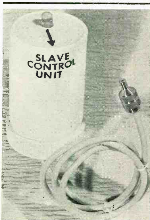
Fig. 3. Light-sensitive end of light-dependent resistor should protrude from one end of plastic container as shown here.
