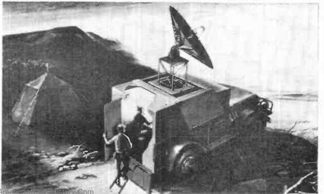
BATTLEFIELD TERMINAL — Mobile communications terminals that provide battlefield commanders with virtually instantaneous worldwide communications via satellites are being developed by Sylvania Electric Products Inc. Each terminal will contain tracking equipment, a control console, a transmitter, and a receiver. It will be possible to transport an entire unit, including a 12' diameter collapsible dish antenna, on a medium-sized truck.
