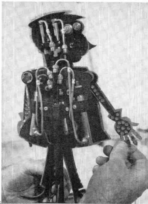
Tape decks control mechanical figures at the IBM Pavilion. Pneumatically-operated puppets, like the one shown below, act out playlets on computer logic complete with sound effects, music, and dialogue.
