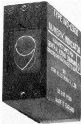
Fig. 12. Each edge-lit plastic strip in the sandwich has a numeral-shaped pattern of dimples on its surface. Photo courtesy of General Radio Co.
