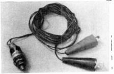
Simple gadget for turning over engine consists of two clip leads connected to normally-open push-button switch. Leads are connected to starter control terminals of starter solenoid.
