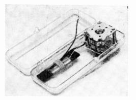
volume control the signal is fed directly to an earphone jack. Additional transistor stages can be added, if desired, to drive a loudspeaker. A patch cord could be used to connect the radio earphone jack to the input of a tape recorder or phonograph. A feedback loop from the detector to the base of the first transistor in the module provides a.v.c. action. Overall gain of the i.f. module is about 55 db.
