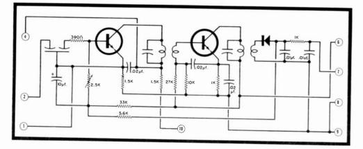
Fig. 6. Miniature i.f. strip is prealigned and pre-packaged. A detector stage is also included. A ceramic filter limits i.f. response to improve receiver selectivity without damaging audio quality. Overall gain is 55 db and output is sufficient to directdrive an earphone. Bandwidth is 8 kc. at-6 db. Photo at right shows how actual components were fitted into can.
