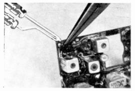
AVOID TOO MUCH HEAT High heat can damage components. Use low heat for soldering, and a pair of long-nose phers to hold the wire. Pliers act as a heat sink and prevent overheating.
