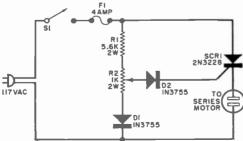
LOW-COST SCR MOTOR SPEED CONTROL
