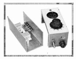
A LTHOUGH the price of speed controllers for power tools has dropped from \$25 to \$10 in the past two years, you can still build your own at a very substantial saving. The "secret ingredient" is a brand-new silicon-controlled rectifier with a 5-ampere rating which sells for \$1.62. It is the RCA Type 2N3228 and is now commonly available either by mail order or from many local electronics stores.
