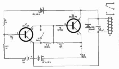
Fig 1. Reader Ronald L. lves employs transistors to latch relays and other control devices. Circuit stays off until triggered by momentarily closing switch S1. Circuit stays on until switch S2 is temporarily opened or until the power is removed.
