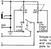
Simple instrument measures values of coils and capacitors. Adjust pots to match voltage across unknown parts.
