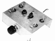
One capacitor, one pot, two transistors, and one resistor add up to a versatile little amplifier. Capacitor C1 should be rated at 50 volts; resistor R2,  $\frac{1}{2}$  watt.
