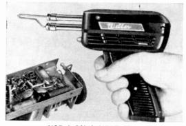
USE A DUAL HEAT GUN A Weller Dual Heat Gun has 2 trigger positions. One provides low heat for electronic connections: the other gives high heat when needed. You switch instantly to the right temperature for the job.
