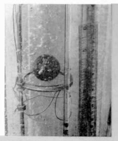
Although lead ball appears to be floating, it is actually riding on a cushion of magnetic force set up by the loop of wire below it in liquid helium. This opposition to any magnetic field is known as diamagnetism.
