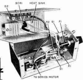
The heat sink in the speed control must be insulated from the aluminum box; use H. H. Smith Type 2645 ceramic insulators Position sink so that it will not short out to the metal back of the outlet.
