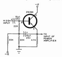
feed the amplifier from a high impedance source. Incidentally, I feel that the regulated d.c. supply is a luxury—any low-impedance 12-volt power supply with a current capacity of 1 to 2 amps will suffice to power the amplifier.
