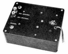
the charger is on or off, it also tells you if the B+ power supply is working up to this point in the circuit. Resistor R2 limits the amount of current that can be passed by the neon light. Output from this half-wave rectifier power supply is approximately 140 volts.
