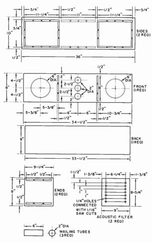
enclosure sections together are made of  $\frac{1}{2}$ "-square stock. Cut enough pieces of the right length for the two sides, and place them exactly as shown in the detail construction drawings above. Secure them in place with glue and screws. Cut the front, back, and ends from ordinary plywood, and fasten cleats to the front and ends as shown.
