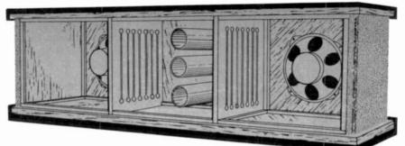
Two-speaker enclosure can be used on its side as above, or on end as seen below. Novel filters (the slotted boards) and ports furnish bass boost.
