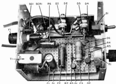
Aluminum heat sink is mounted to one side of box on a Bakelite strip; PC board is mounted on  $\frac{1}{2}$ " spacers. Only rear of SO1-the socket for lights-is seen. Heat sink and components should not contact metal box.
