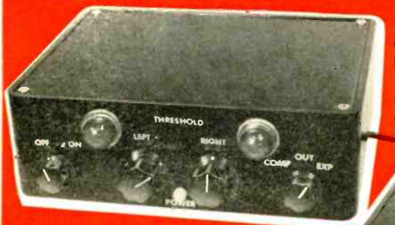
Controls on front of unit (photo above) are threshold controls which determine the level at which expansion or compression takes place. Panel lamps I1 and I2 glow in proportion to the voltage of the audio tapped from speakers; switches control power, function.
