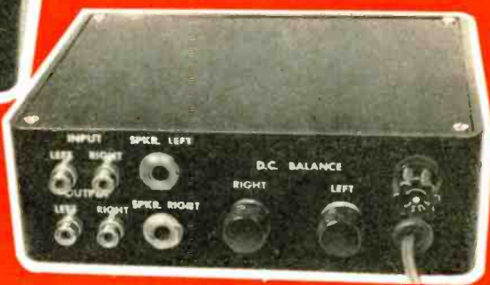
Controls on front of unit (photo above) are threshold controls which determine the level at which expansion or compression takes place. Panel lamps I1 and I2 glow in proportion to the voltage of the audio tapped from speakers; switches control power, function.
