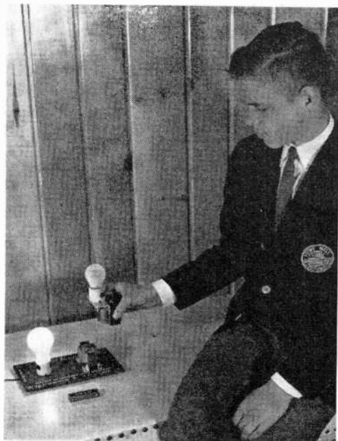
Fig. 1. Operator removes flux link from choke L_1 , reducing inductance of the choke and causing series-connected, 60-watt lamp L_1 to glow brightly.
