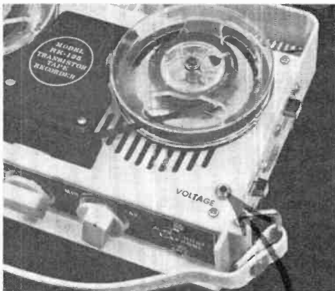
Subminiature jack (J2) for monitoring battery voltage can be installed on top of panel.
