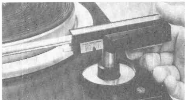
The M232 arm is statically balanced by a counterweight which is adjusted by knurled knob under arm. Tension is set by spring adjustment to 3 grams.
