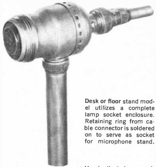
Hand mike below, a variation of the unit above, is turned on and off by original lamp-socket switch. See construction details at bottom of page.
