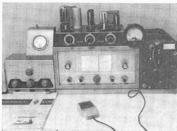
A hi-fi amplifier can be used as a modulator by connecting a replacement output transformer back-to-back with the amplifier output transformer as shown in the diagram. Jeff Binckes, K9OLL/8, uses a Heathkit amplifier (left) to modulate his AR-3 receiver, as described in the text.
