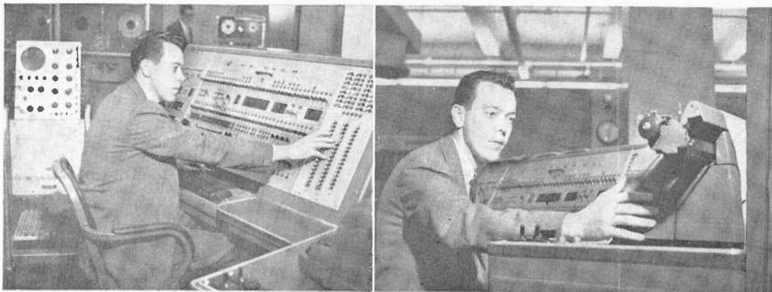
When trouble-shooter Jim Stewart starts to work on a computer, he first programs some tests on the control panel (left). Then, he checks results of tests on read-out typewriter. In many cases, this gives Jim enough information to deduce which circuit is causing the difficulty.
