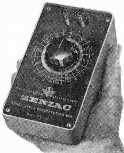
Fig. 2. How a Zener diode is used as a voltage regulator. See text. International Rectifier's new Zeniac substitution box, shown above, offers a selection of 11 basic one-watt silicon Zener diodes from 3.6 to 30 volts.
