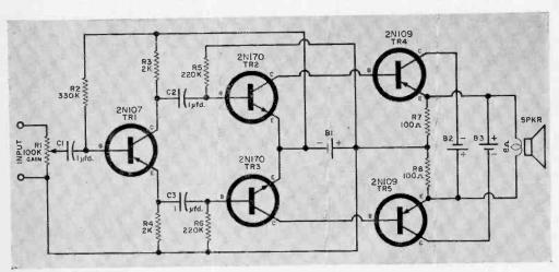
Fig. 1. Reader Lee Baker's five-transistor audio amplifier requires no audio transformers, yet provides good gain.
