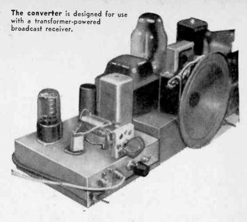
caution should be taken. Locate the input circuit (L1) and (L1) away from the oscillator tank circuit (L4), (L4), (L4), and away from the output coil (L2). Note that the input coil and capacitor are mounted on top of the chassis and the two other coils are underneath and spaced from one another.
