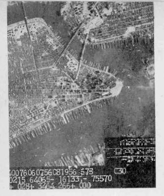
A camera writes its own captions! The illustration above shows how position, altitude and other pertinent data necessary to Air Force reconnaissance can be recorded automatically on photos. Developed by Federal Telecommunication Labs, the Digital Data Recording Device records all data in coded dot form (lower right on photo). During development, a ground-based reader decodes and prints data under picture.
