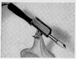
and the heavy metal base anchors it fast. Secure the clip to the base with a machine screw and wing nut through the clip's handle. Bend the jaws, if necessary, to receive the iron's barrel.
