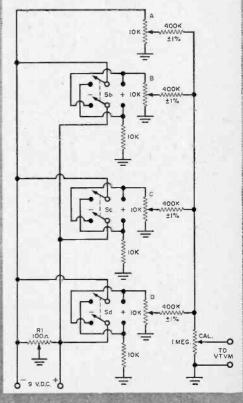
Fig. 4. Four-number adder-subtracter unit.
