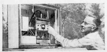
Data is picked up by Geiger counter (being installed in snow gauge in top photo) through the snow from a tube of cobalt 60 directly below it. At left is receiver and transmitter at base of gauge. The radiation data is automatically transmitted to a Corps of Engineers' receiving station.
