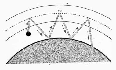
Fig. 3. When the satellite was below the ionosphere, Russian listeners heard reflected signals at times.
