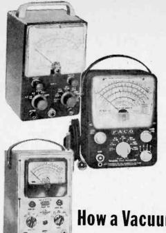
THE ACCURACY of any voltmeter reading depends upon the extent to which it affects the circuit under measurement. After the voltmeter is connected, the voltage no longer has the same value it had before the instrument was attached.
