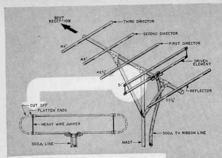
performance is dependent upon a combination of factors, such as interelement spacing, element lengths and diameters. Since these dimensions vary from one make of Yagi to another, a general procedure applicable to all antennas of this type must be employed.
