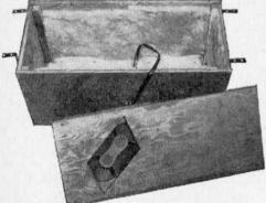
The speaker can be seen through the parallelogram opening. While it's not evident above, the speaker is actually mounted on a board separated from the front panel by two spacing blocks made of pine.
