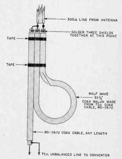
Fig. 5. Balun transformer at receiver provides an impedance change of 4:1 and is used to connect a balanced termination to an unbalanced one.
