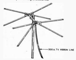
their resonant frequency from channel 6 (about 83.25 mc.) to the satellite channel. A few minutes work with tin snips or hacksaw can complete the job. Trim equal lengths off the tips of each element to change the operating frequency. The new over-all dimensions (tip-to-tip) for a 5-element array are shown in Fig. 3.
