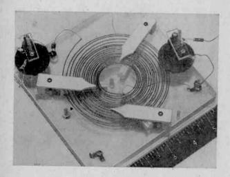
The "watchspring" above is actually a torsional delay line, a device used in such applications as computer work, trigger-delay circuits and radar range measurement. Developed at Bell Telephone Labs, it is made of Vibralloy, a ferromagnetic alloy. The spiral permits clear resolution of 10-microsecond pulses spaced 20 microseconds apart.
