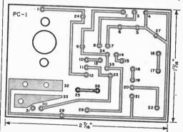
you can add 25 and 26 by drilling two  $\frac{1}{16}$ " holes in the proper positions and installing a short length of wire between them.
