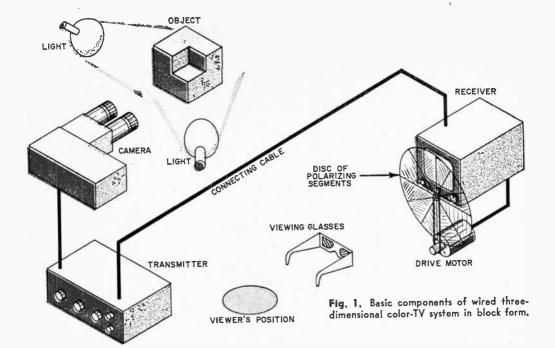
polarized. The special viewer used by the observer is equipped with one filter for each eye, which sees only the image meant for it, with each image retaining the full color of the original scene. It is this system, used in 3D motion pictures, that has been adapted to 3D color television.
