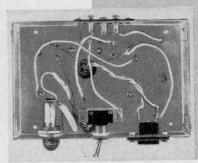
Fig. 1. Power transistors in oscillator circuit (on page 36) operate from 12-volt battery.
