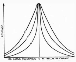
member about Q are the above formula and the fact that a high-Q circuit has high selectivity. The resonant circuits in our transmitters normally should have an effective Q of at least 10 for sufficient selectivity to suppress harmonics and other undesired frequencies unavoidably gener-
