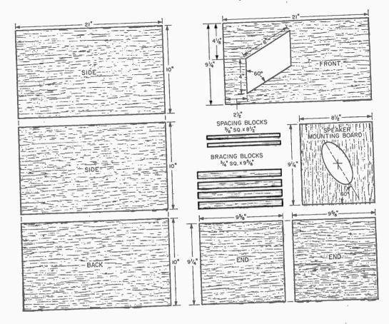
tion is used on the front panel or the end nearest the speaker. Insulation is required on both sides, the back, and the end farthest from the speaker.
