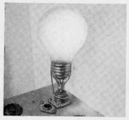
strips comprising the shell of the connector apart and solder them to the lamp base as shown. Then solder a piece of #12 copper wire to the lamp base and extend it to form a circle around the connector pin. It should fit snugly around the barrel of the transmitter's coax connector.
