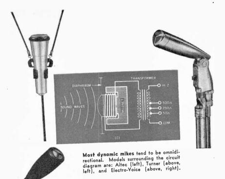
250, 500 ohms, or even higher, to match the amplifier input. Such transformers are generally tapped to allow selection of any popular impedance. In one instance, that of the Altec 633A, the voice coil (30 ohms) is used directly to feed a 50-ohm amplifier input.
