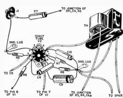
be used as either a self-contained radio or as a tuner for your hi-fi system. Capacitor C7 is connected from the "high" side of volume control R2 to this jack. Since the audio output signal of the tuner is not affected by R2, this permits the exclusive use of the volume control on your hi-fi amplifier for controlling the tuner.
