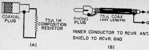
Fig. 5. Dummy load (A) for adjustment and interconnecting cable (B).
