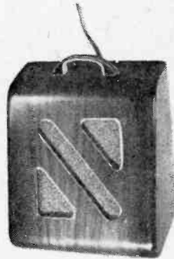
Several typical p.a. components are (top to bottom) a University reflex trumpet, dynamic Electro-Voice cardioid mike, controlled-magnetic Shure omnidirectional mike, and cone speaker in standard wall baffle.
