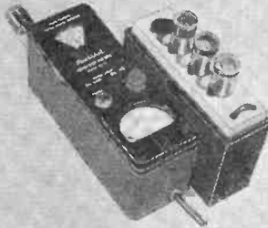
GRID DIP METER
