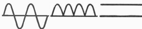
Fig. 1. Rectifier changes a.c. to pulsating d.c. inductor a useful complement to the capacitor in a power supply filter circuit.
