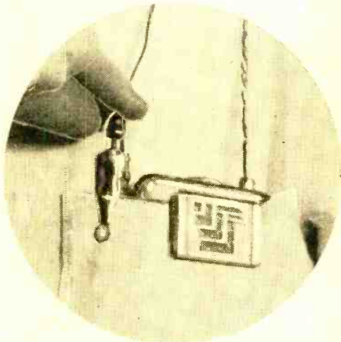
The converted unit mounted in a shirt pocket, and being tuned by adjusting the loopstick screw.
