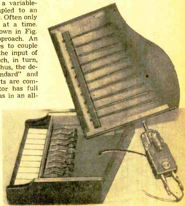
Fig. 8. Interior view of the toy piano, with an enlarged view of the phonograph pickup used to pick up the vibrations of the sounding pins. The pickup can be located approximately in the position indicated by the arrow, but exact position should be determined experimentally so that optimum volume and tonal quality are obtained from the instrument.
