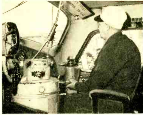
The operating position in a diesel. Note how the handset for the two-way radio is mounted so that engineer can reach it from his chair.
