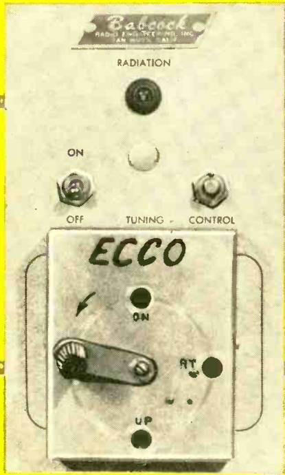
Fig. 1. Rotary ground control switch added to a Babcock transmitter. The regular control button of the transmitter serves as the sync button.
