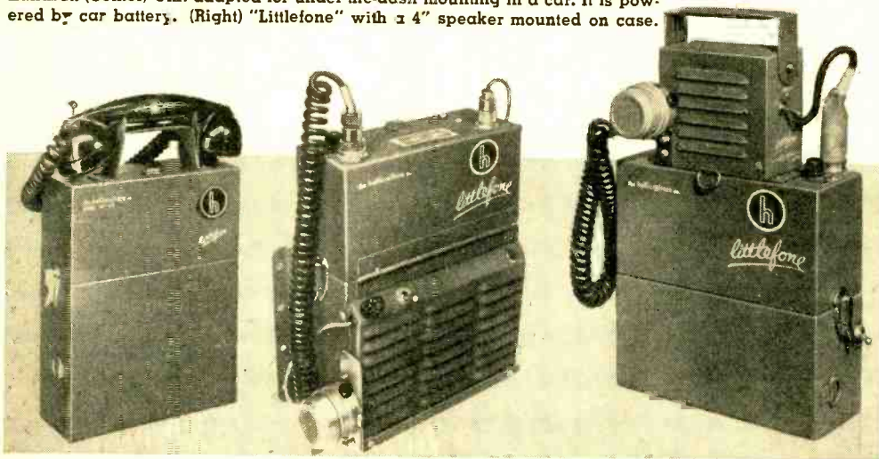
Three versions of the Hallicrafters "Littlefone." (Left) The standard model with handset. (Center) Unit adapted for under-the-dash mounting in a car. It is powered by car battery. (Right) "Littlefone" with a 4" speaker mounted on case.
