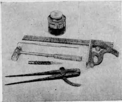
Tools needed for laying out chassis: dividers, center punch, small hammer, scribe, combination square, and can of layout fluid.
