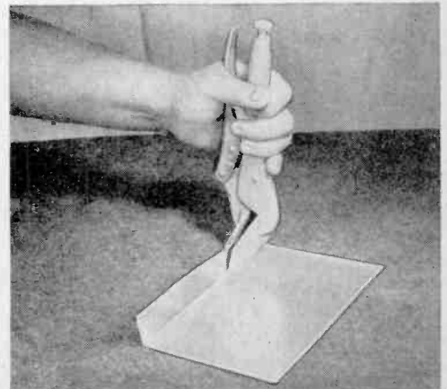
Fig. 7. Using the same special tool to bend a larger chassis by making repetitive bends.
