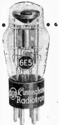
Fig. 3. The electron-ray tube, in many applications, replaces a more delicate meter.
