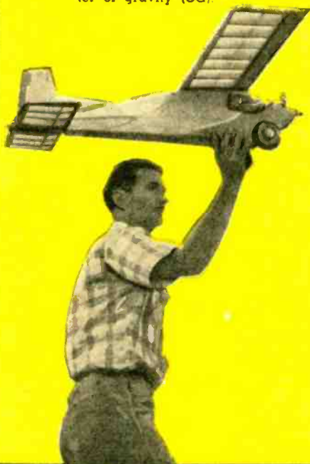
Fig. 3. For the test glide, hold the plane under its center of gravity (CG).
