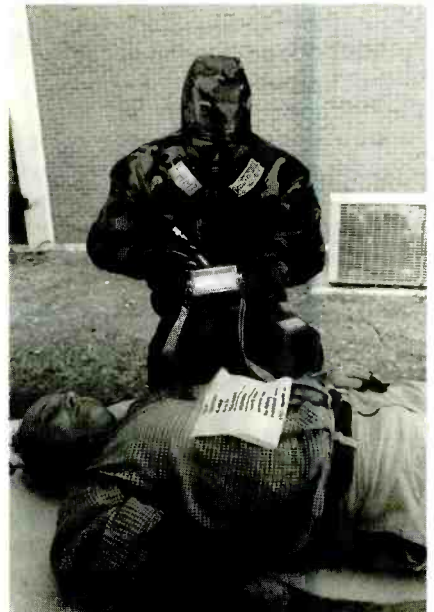
A first responder goes through an electronic checklist of symptoms using ChemBio Decision Aid software running on a PDA. (GTRI photo by Stanley Leary.)
