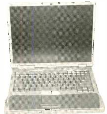
Hewlett-Packard's Omnibook 6100 is a full-size two-spindle notebook with a 15-inch screen. Features include both a touch pad and a pointing stick.
