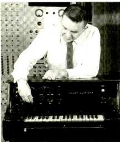
Scott with his 1950's keyboard synthesizer invention, the Clavivox.
