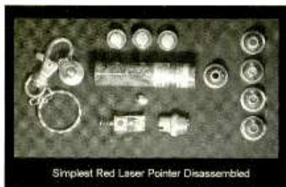
Here's what you get when you crack open one of those bargain laser pointers. As you can see, the parts are minimal—power source, driver, laser.
