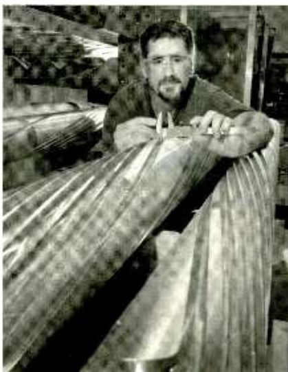
A specialized set of magnets called Siberian snakes were built. Their corkscrew-like design causes the direction of the magnetic field to spiral along the direction of the beam.
