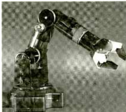
Here is the OWI Robotic Arm Trainer that is controlled via a PC interface. What makes the arm suitable for computer control is the fact that it uses five small DC motors to produce motion in the base, shoulder, elbow, wrist, and gripper.
