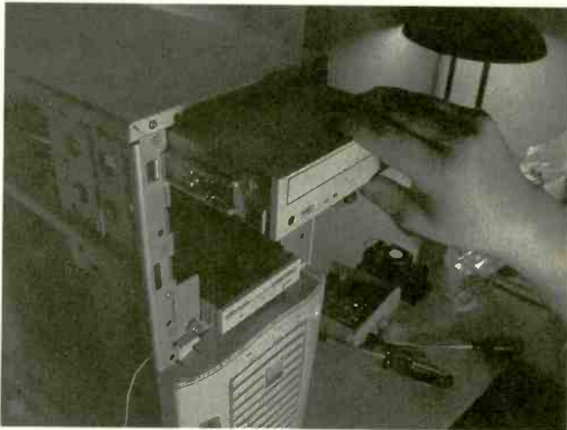
Photo 10. Slide the drives into the case, as shown here.
