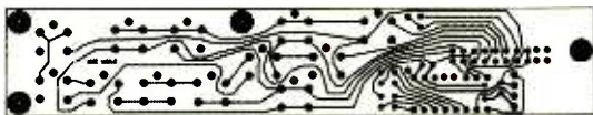
Fig. 10. Here is the solder-side foil pattern for the pushbutton board. A high-resolution image can be downloaded at www.pjrc.com/tech/mp3/pcb_layout_reva.html .
