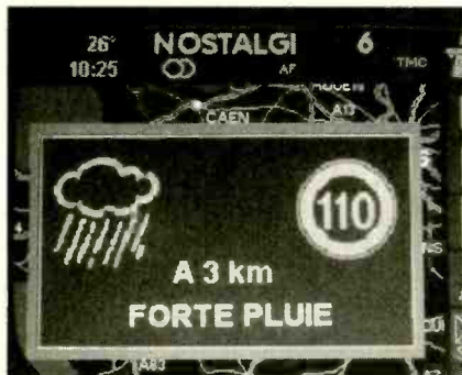
On the AIDA screen, icons or short messages display information about road hazards.
