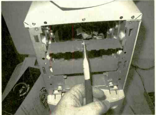
Photo 7. A pair of pliers is used to remove knockouts where the two optical drives will go, as shown here.
