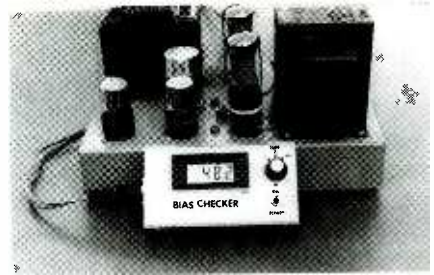
The completed Tube Amplifier Bias Checker is a welcome addition to any audio technician's toolbox.
