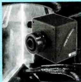
Shown here is an OPSIS 5150 camera juxtaposed against a background of a molten-glass stream.
