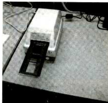
The film or slide holder is then placed into the slot in the scanner's front panel, and the TWAIN driver is launched to perform the scan.
