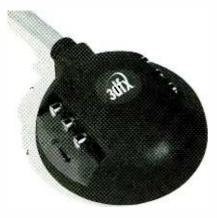
Except for cable TV and FM antenna, connections to the 3500 TV are made via the innovative I/O Pod shown here. Forget about reaching behind your PC to work with video sources.
