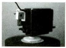
Fig. 4. This servo has been modified with a small 5000-ohm trimmer potentiometer to replace the one removed from the servo. It is mounted to the outside of the servo case with double-sided tape. The potentiometer allows easy calibration to find the servo's center, or neutral, position.
