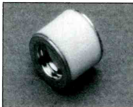
Figure 5. Gas tubes incorporate a gas-filled gap that offers high resistance to normal operating voltages. When the voltage becomes high enough, it starts conducting and shunts the over-voltage safely to ground.
