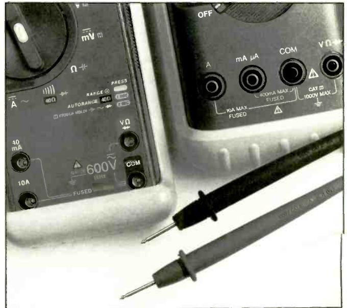
Figure 6. Look for category and voltage ratings of test leads and multimeters.
