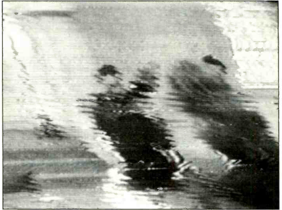
Figure 1. When I first operated the Hitachi model VT-M241A to evaluate its condition, it produced this wavy picture.
