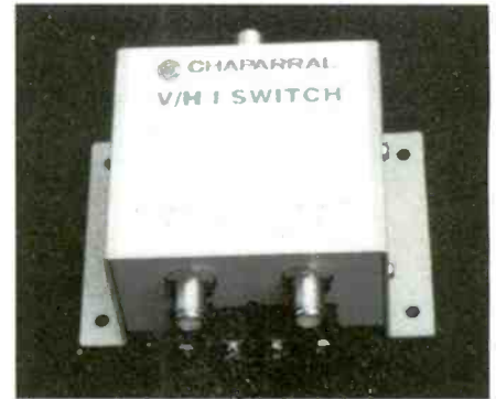
Figure 7. If the IRD in the system you wish to convert from C-Band to Ku-Band has only one IF input, a separate coax switch is necessary.
