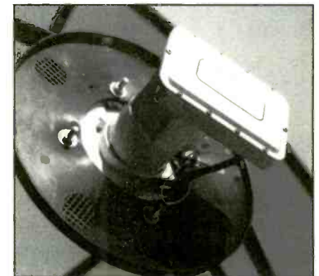
Figure 8. If the C-Band system has an LNBF (an LNB combined with a feedhorn), you will have to order a C-Band LNB with a noise temperature of 20K.
