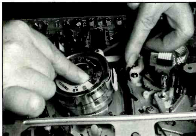
Figure 4. Cleaning the video heads
